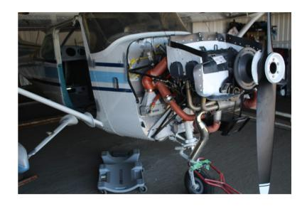
Inspection of the air frame: Removed interior, doors, rear window, headliner and inspection covers.
