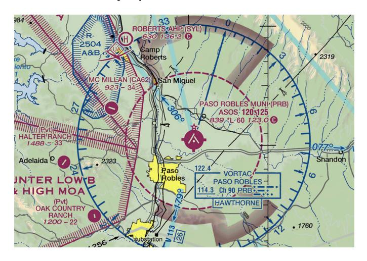
The name of the airport in the center of the image is Paso Robles Municipal. The code is PRB. There is no control tower, indicated by the magenta airport circle enclosing the runways. The star on top of the circle indicates that there is a rotating beacon. The Common Traffic Advisory Frequency is 123.0. ATIS is 120.6.
